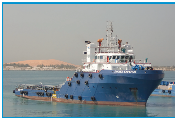
61M 5150 BHP OFFSHORE SUPPORT VESSEL (DP1, FIFI 1)
